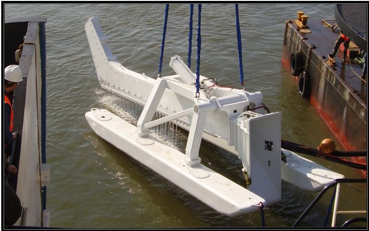
FIGURE 2-10: PHOTOGRAPH OF A TYPICAL JET PLOW
