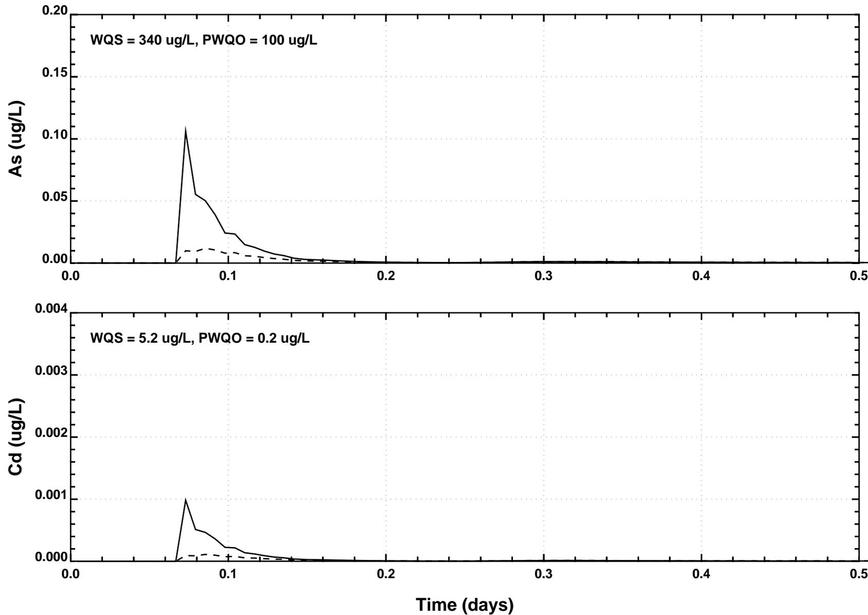
**Figure 67. As and Cd Model Projection Results at KM70**
